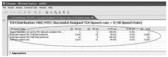
Chart shows the effect of half rate not being enabled.
